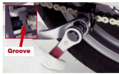
**11a.** Hold the hexagon part of the tool body with a 27mm closed end wrench and turn the bolt with a 19mm closed in wrench clockwise until the top of the pins make contact with the groove in the Plate holder.
