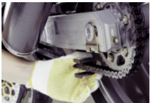
**1a.** Before cutting your chain, loosen it using your motorcycle's rear wheel adjusters. Position your KM500R or KM501E over your chain on the bottom side of your swingarm; cut the pin on the right side of the link you choose first. If your chain has a master link, it is easier to cut the chain at the master link.
